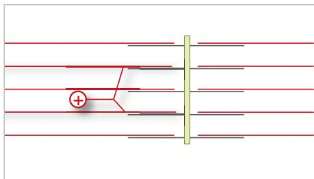
3. At each of the edges towards the Egcobox®, there must be one marginal strip provided in accordance with EN 1992 (min. dim. stirrup  $\varnothing 6 / 250$  mm plus  $2 \times 8$  mm bars parallel to joint). On the balcony side, the marginal stirrup should at least correspond to number and diameter of the shear force bars of the Egcobox® element.
